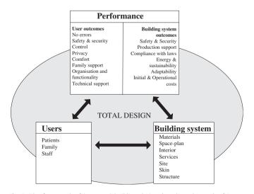
Fig. 2. The framework of integrated building design, based on the work of Rutten [1996] and Ulrich et al. [2004, 2008].
